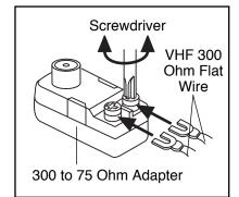
2. Connect the 300 to 75 ohm adapter to the 75 ohm antenna terminal on the treadmill. (See assembly drawing 5 on page 8 to find the location of the terminal.)
